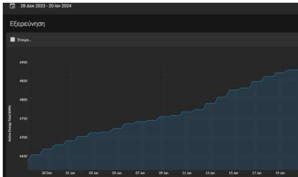
Figure 63. Electric production from PV (panels of 6KW-monocrystalline) monitored by PragmalIoT. PS#5
