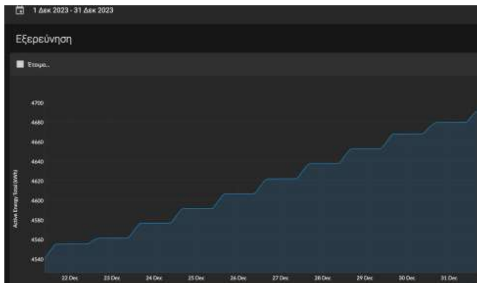
Figure 62. Electric consumption kWh (UPS loads in 1st floor offices) monitored by PragmaIoT (21-31 December 2023). PS#1
