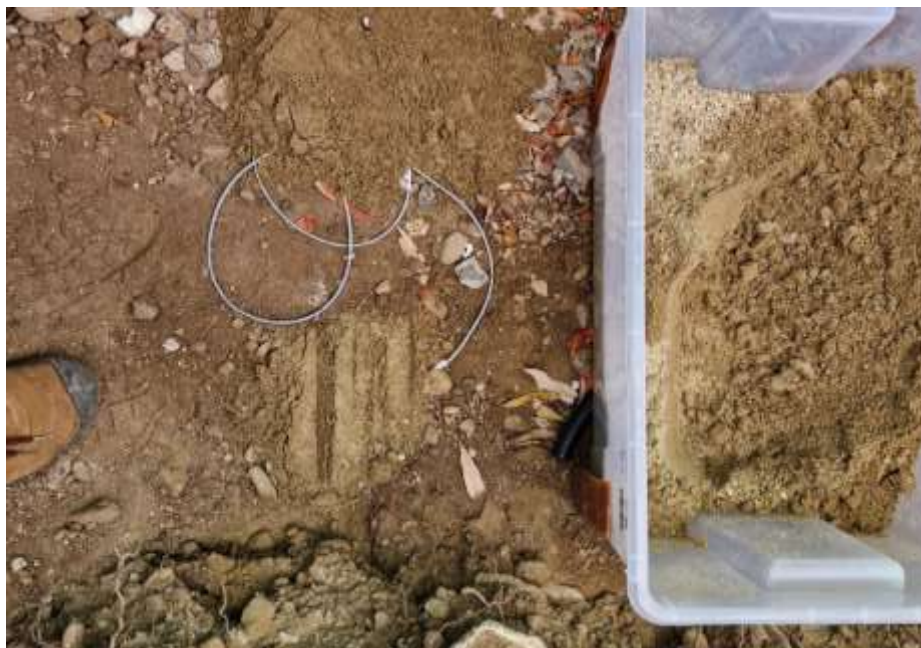
Figure 19. Ground temperature sensors installed
