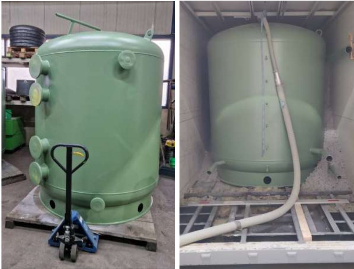
Figure 51. Buffer tank and insulation process of the DH-buffer tank
