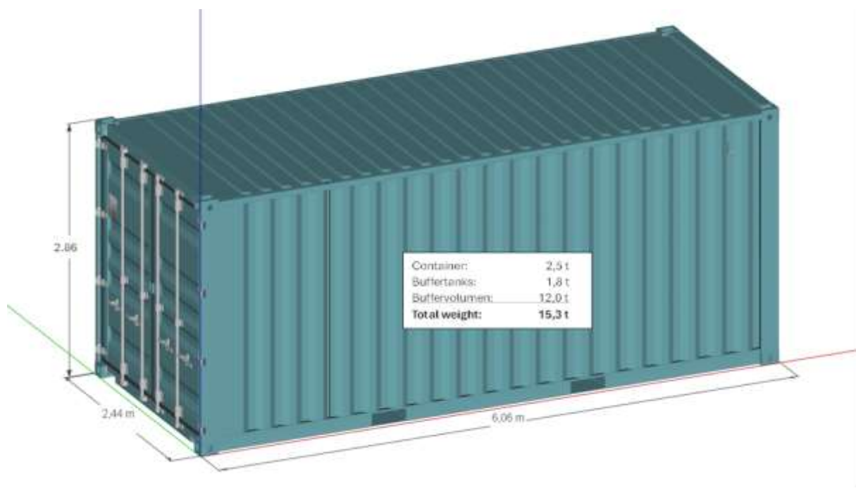
Figure 47. Dimension and weight of DH - buffer tank
