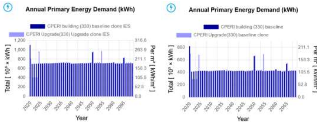
Figure 56. Lifetime Primary Energy Demand for the baseline scenario (left: iSCAN-approach, right: INTEMA-approach)
