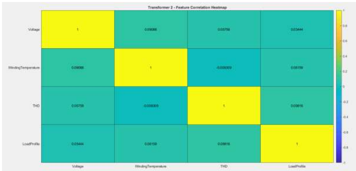
Figure 18. Correlation heat map for key transformer 2 parameters
