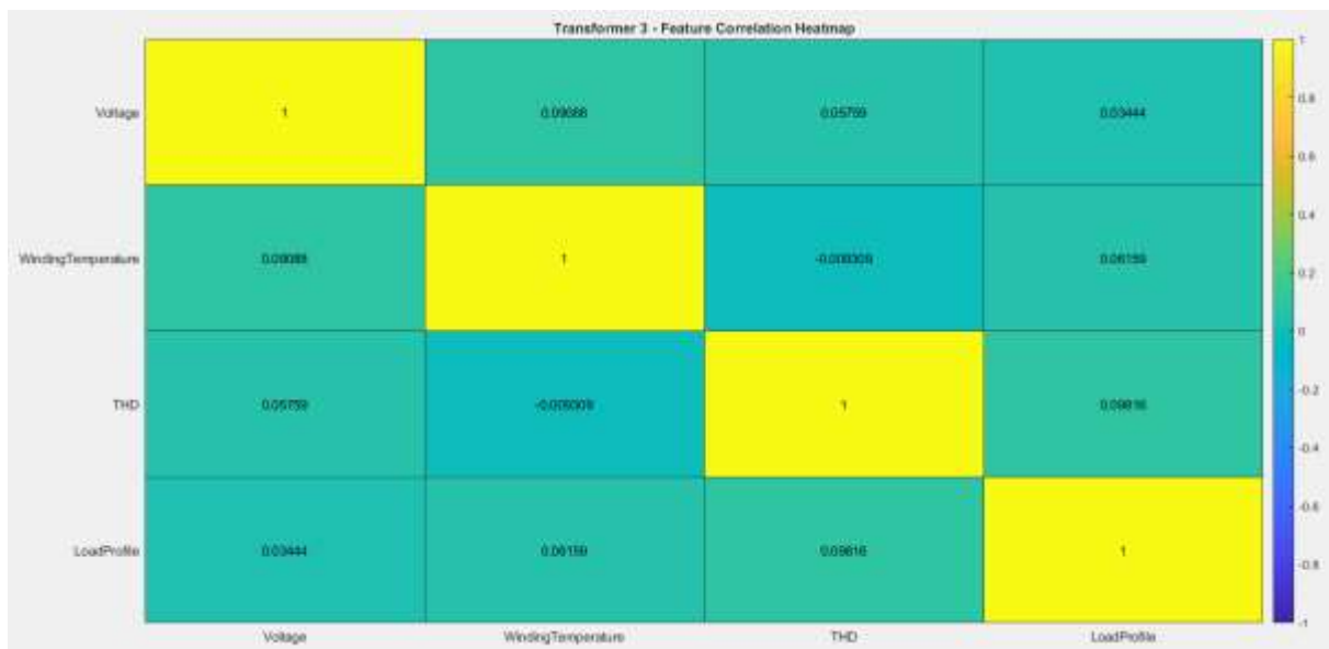
Figure 19. Correlation heat map for key transformer 3 parameters
